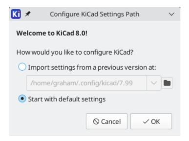
If a previous version of KiCad is detected, you will have the option to import the settings from that version. The location of the previous configuration files is detected automatically, but you may override it to choose another location if desired.
