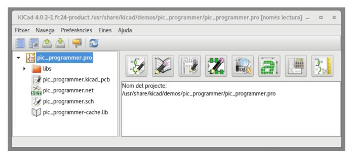
The KiCad project manager window is composed of a tree view on the left showing the files associated with the open project, and a launcher on the right containing shortcuts to the various editors and tools.
